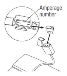
3. Remove any fuse that is damaged or burnt out and replace with a new one of equal amperage.
