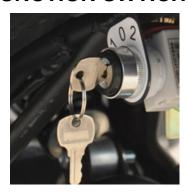
The 3-speed limit key is located under the right side of seat (see above pictures). There are 3 letter standing for the different speed as follows:
