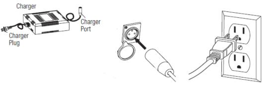
1 Turn OFF power switch before charging. Plug charger into the charger port on the electric motor bike.
