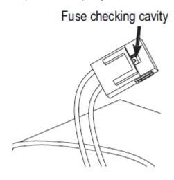
2. Check the fuse to see if it has burnt out. If the fuse is damaged, open the fuse cover.
